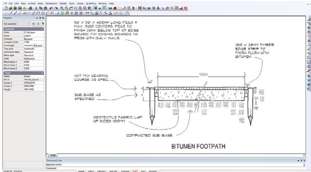
It is possible, but not normal desirable to override dimension value. In this can the path section has been broken and the path width is shown as 1000 using an override.
