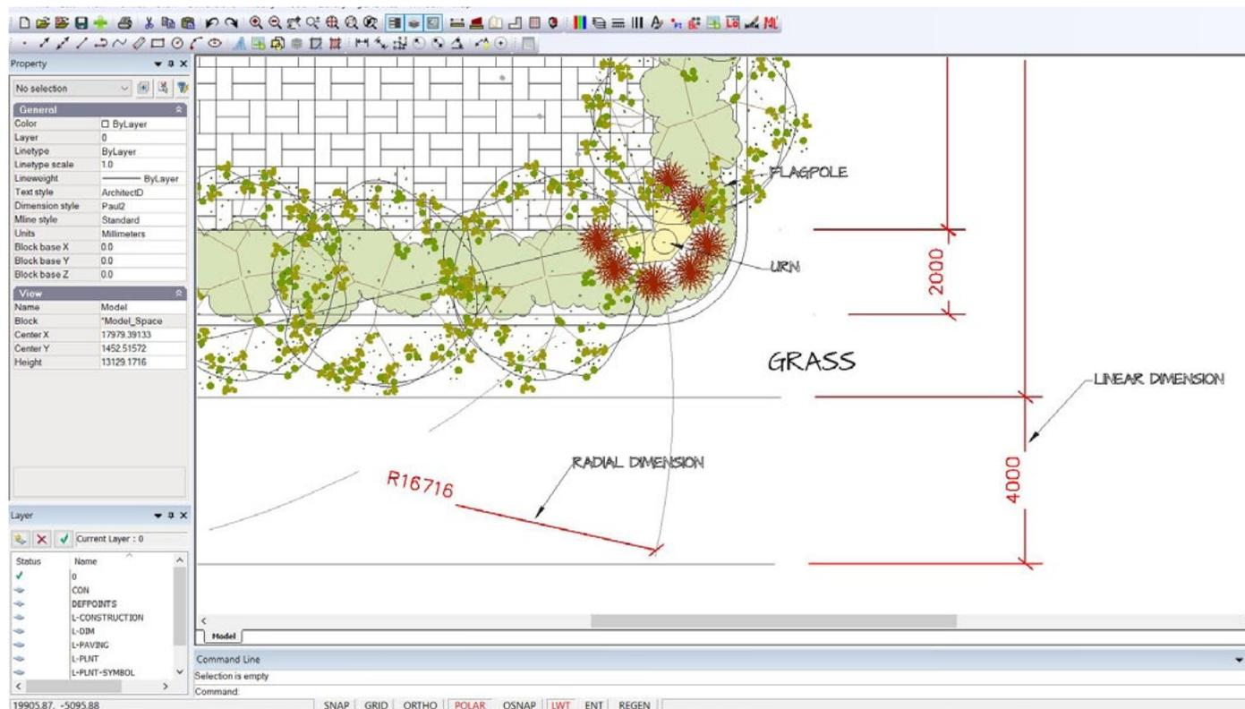
Some examples of dimensioning applied to a gCADPlus drawing. The dimensions have been placed on their own layer so they can be displayed in a layout space.
