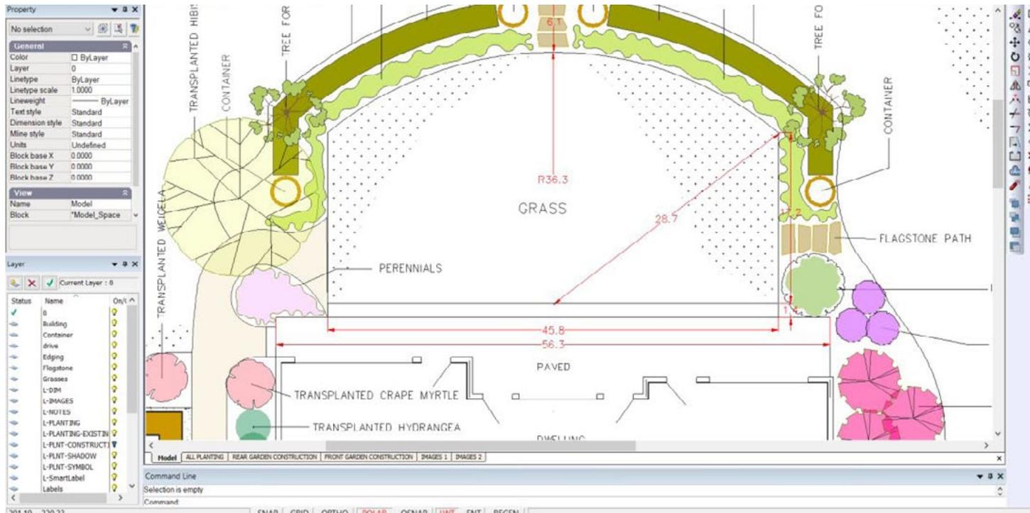
An example of dimensioning in a gCADPlus design from the USA. Here the base drawing unit is decimal feet. If needed, the dimension style can be edited to display dimensions as feet and inches.
